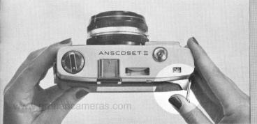
The film rewind knob (No. 1) should turn counterclockwise as the film is advanced; if it does not, it indicates that the film was not properly attached to the take-up spool. Open the camera again and reconnect the film, making sure that the film is taut and that the sprocket teeth are engaged in the film perforations.
